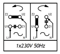
The above diagrams are only a connection guide. The correct wiring diagram for a particular motor model is located under the terminal box cover. The above diagrams do not include sensor connections that may exist in specific device versions.
